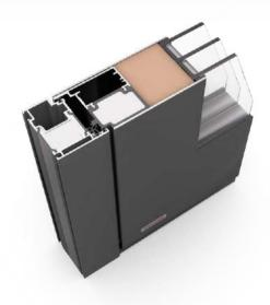
$U_d$  (thermal transmittance) = 0,71 W/m<sup>2</sup>K Cylinder length inside / outside: 35/50 mm Door frame width 75 mm Door Leaf width 89 mm Triple glazing RC2, RC3 Certificate (surcharge)
