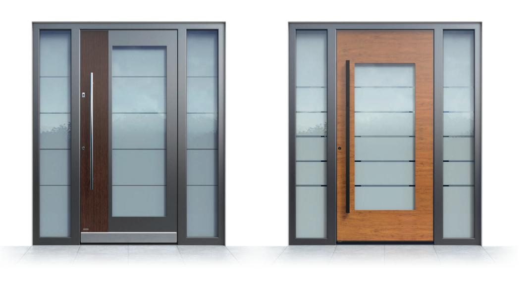
Colour 70105 / Additional decor outside BLACK OAK / Clear glass motif sandblasted / Handle ROUND115 / Reliable locking system with SECURO finger scanner and ARMO COMFORT ELECTRO lock / Stainless steel protective trim 6203
